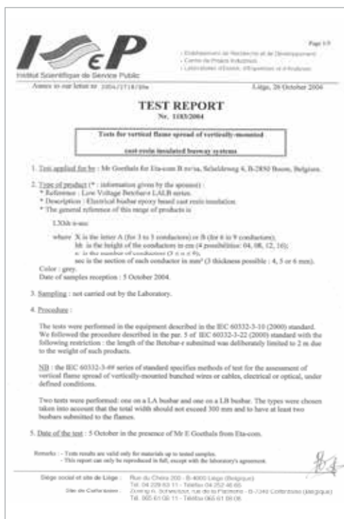
Flame Spread Test as per IEC 60332
